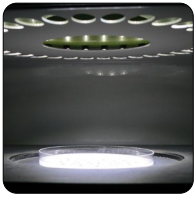
Dark Field: LED are disposed in a circle for optimal contrast
