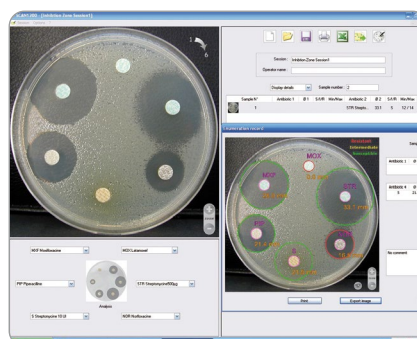
Precision of inhibition zone radius measurement from paper discs: 0.3 mm
