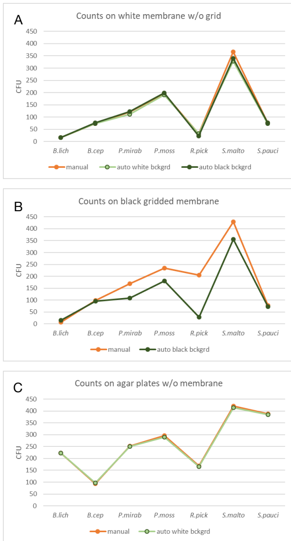
Figure 1. CFU counts of 7 bacterial strains on different types of membranes (A: white membrane w/o grid, B: black gridded membrane) and on agar plate without membranes (C). The orange lines are for manual plate counts ("reference") and green lines are for automatic counts performed by the ScanStation®. For automatic counts, two configurations for light to take pictures were tested: black bckgrd (black background) and white bckgrd (white background). List of bacteria tested= B.lich. : Bacillus licheniformis , B.cep : Burkholderia cepacian , P.mirab : Proteus mirabilis , P.moss : Pseudomonas mosselii , R.pick : Ralstonia pickettii , S.malto : Stenotrophomonas maltophilia , S.pauci : Sphingomonas paucimobilis .
